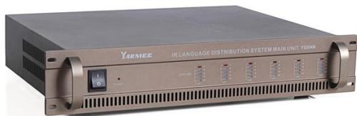
The YS-504M Digital Transmitter is the central modulator unit in the digital infrared system. It accepts audio from the YS-504M or other compatible audio sources. The YS-504M modulates the incoming audio signals onto carrier waves, which are sent directly to one or more YS-504X Digital Infrared Radiators. The output from the radiator is then passed on to each YSN504R delegate receiver.
